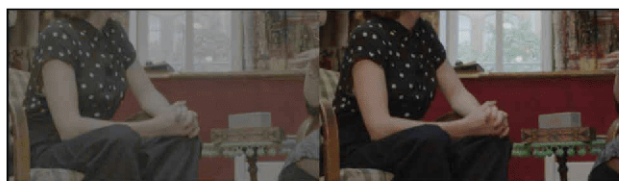
FIGURE 10. Exposure-corrected SLog3 image (left) and the resulting, noisy BT.709 output (right).
