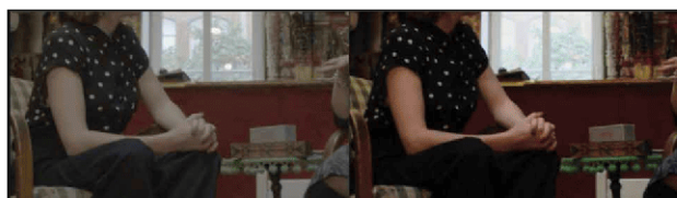
FIGURE 9. Under-exposed section of a SLog3 image (left) and the resulting BT.709 output (right).
