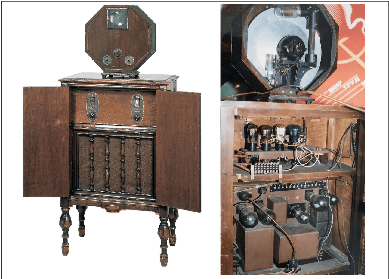
FIGURE 4. (a) “Telopticon” on top of the television receiver contains the neon tube, the disk with a spiral of 24 holes, and the drive motor. The cabinet below houses the receiver as well as the system power supply. “B” is shown to contain the short-wave receiver for the sound portion of the program as well as power supply and loud speaker. (b) Telopticon and receiver, rearview. The neon lamp can be seen, horizontal, at the top. The 24-hole disk and motor below. The broadcast band receiver underneath with the power unit at the bottom. Compare to Sketch A in Fig. 3. (Courtesy of the MZTV Museum of Television.)
