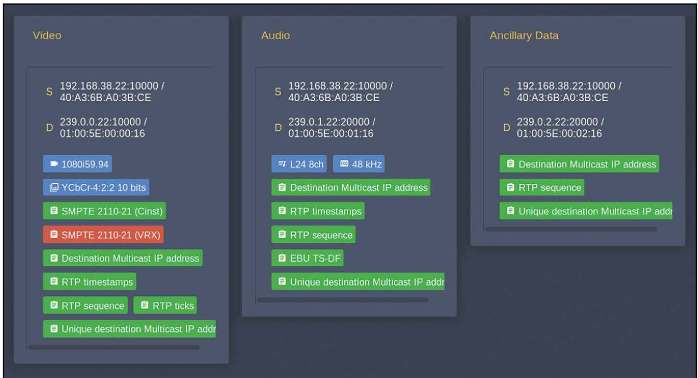
FIGURE 7. Virtual Receiver Buffer (VRX) error visualized in the web graphical interface.
