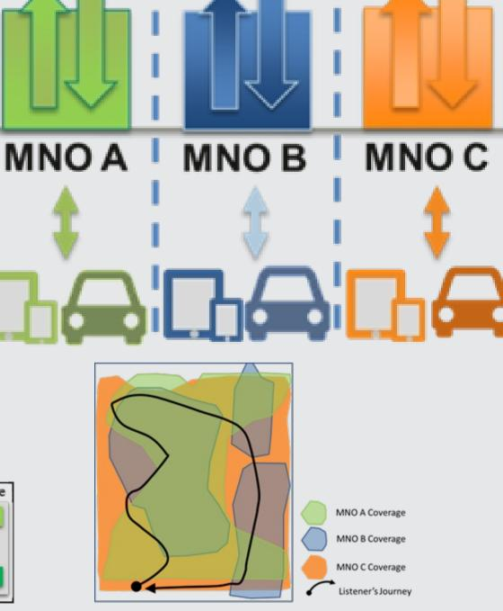
Figure 12: Conventional mobile network operation showing different coverage per operator
