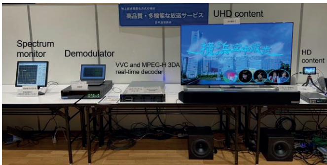
Fig. 2. Equipment of the receiver site
