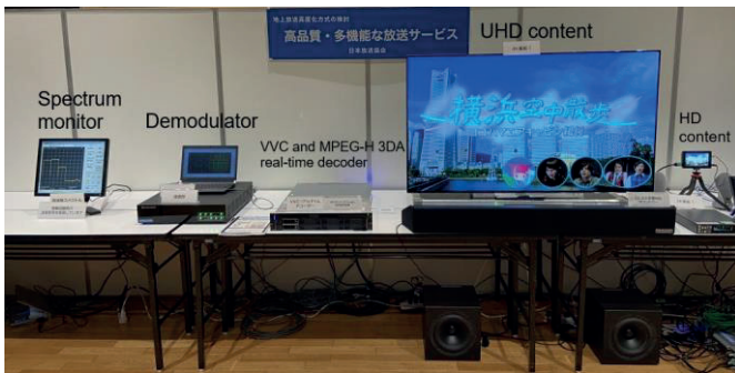
Fig. 2. Equipment of the receiver site
