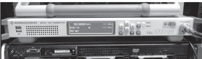
Figure 6. Rohde & Schwarz SFE100 Test Transmitter used to generate noise and mimic real transmission conditions in the experiments.
