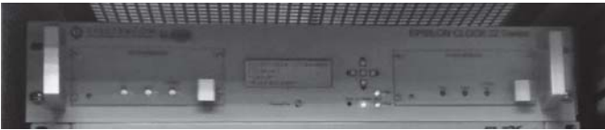
Figure 4. EC225 GPS clock and frequency references generator.
