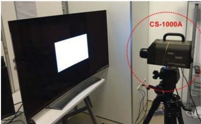
Fig. 1. Position of CS-1000A, perpendicular to an OLED television set.
