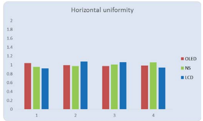
Fig. 8. Results of the horizontal luminance uniformity test.
