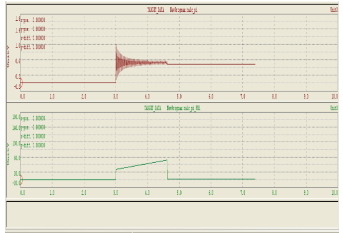
Figure 3. Filter having modified Hamming window in the time domain.
